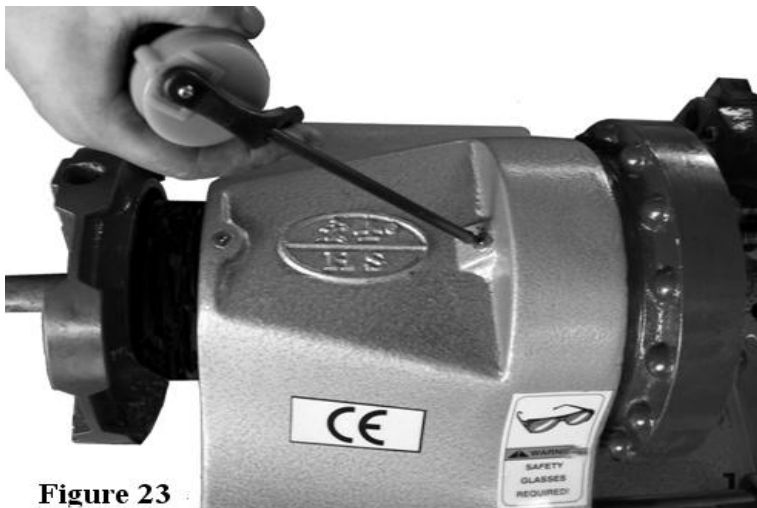
Figure 23. Location of headstock oil ports
