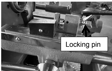
Figure 7. (Slamming hammer chuck to lock it on the pipe)
