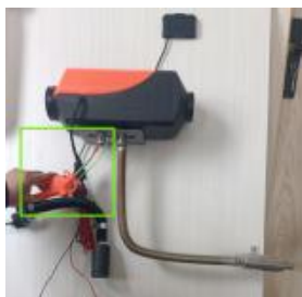
Blow the air gun towards the intake pipe to assist combustion
