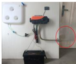
Excessive pump oil produces white smoke
