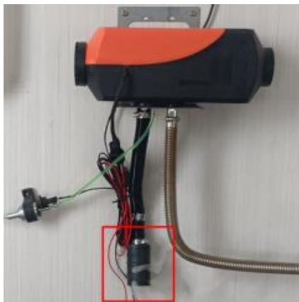
Abnormal power outage and smoke coming from the intake pipe
